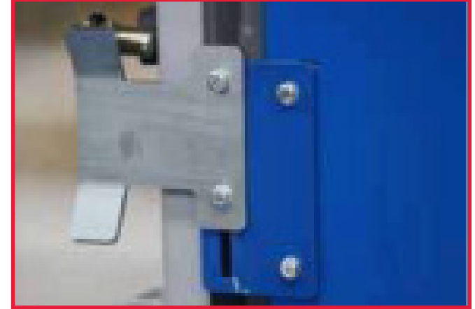
b ELECTRICAL MICRO-SWITCH Emergency function that will stop the platform from operating in an emergency situation.
