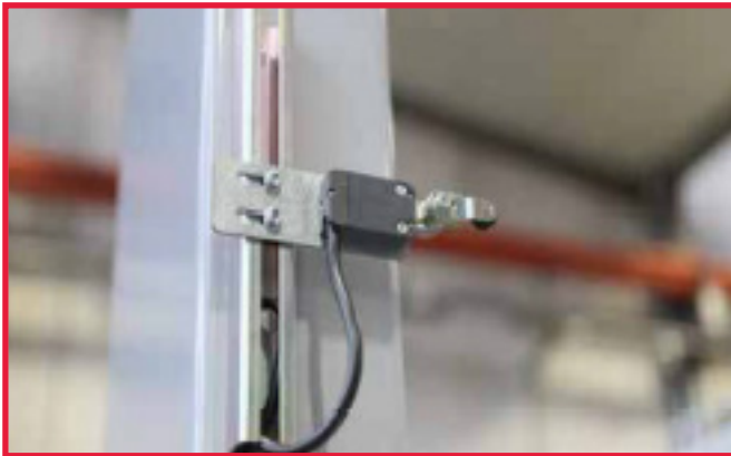
b ALL MICRO-SWITCHES All micro-switches are placed along the column with the possibility to be adjusted by moving positions along the regulation bar.
