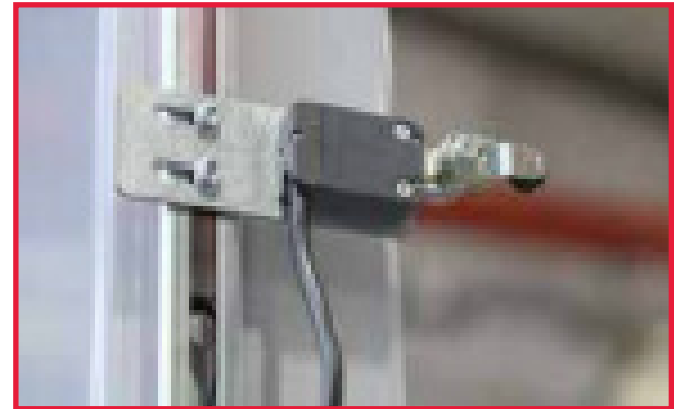
b ALL MICRO-SWITCHES All micro-switches are placed along the column with the possibility to be adjusted by moving positions along the regulation bar.
