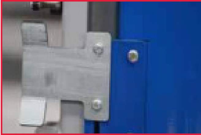
b ELECTRICAL MICRO-SWITCH Emergency function that will stop the platform from operating in an emergency situation.
